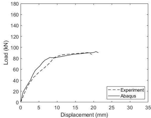
Figure 10. Numerical validation of double shear lap test model
