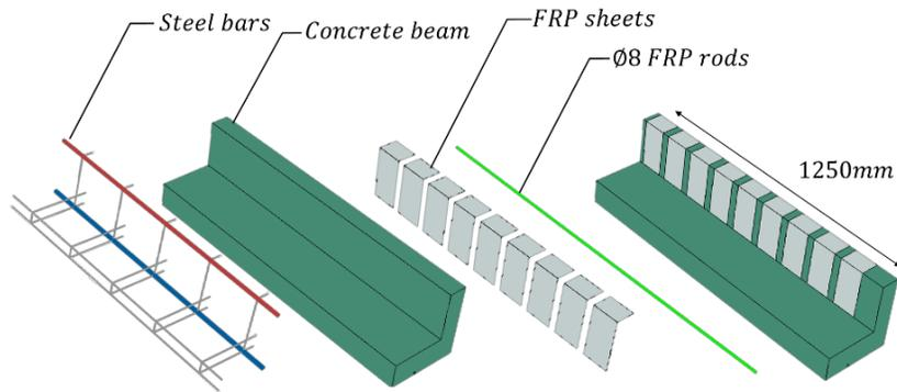
Figure 8. Geometry of 3-point bending test model
