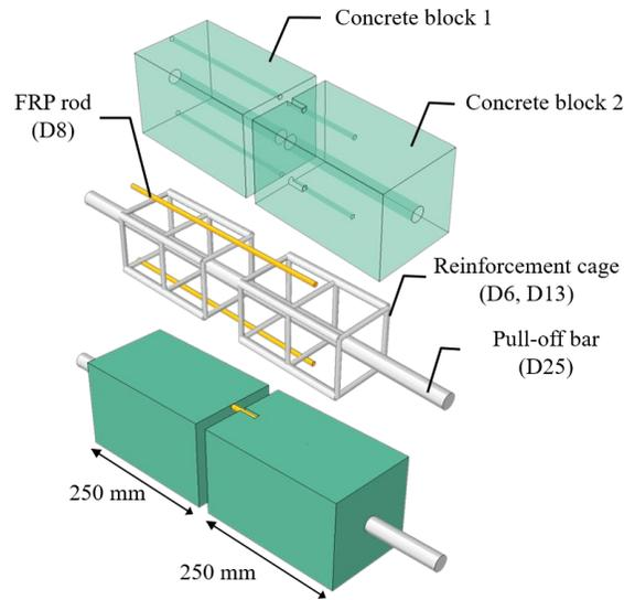
Figure 7. Geometry of double shear lap test model
